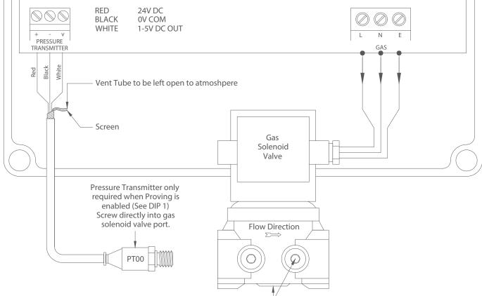
Pressure Transmitter MUST be connected to a DOWNSTREAM port.-
